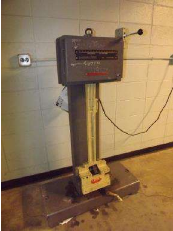
Figure 13: Charpy Impact Tester (mfg. by Tinius Olsen)
