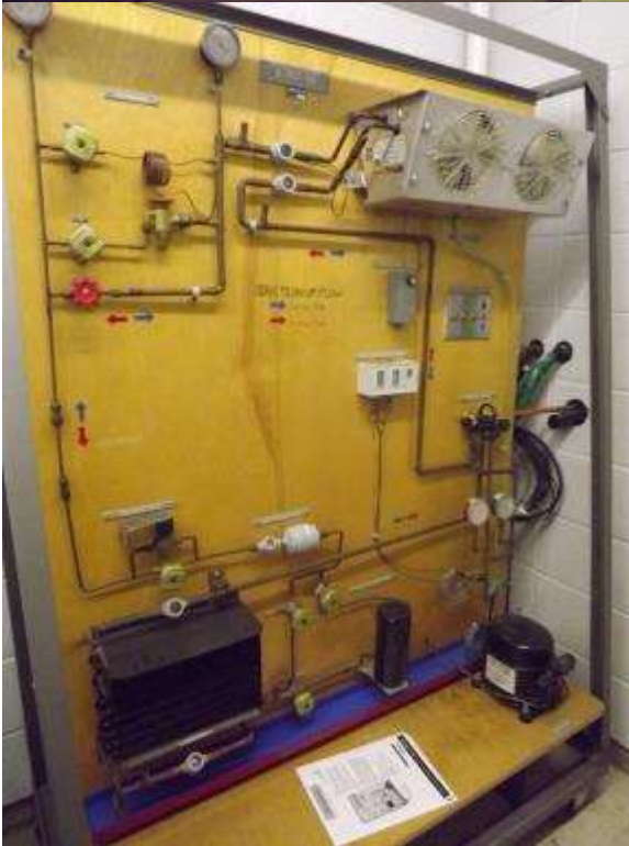
Figure 1: Hampden Refrigeration System Trainer
