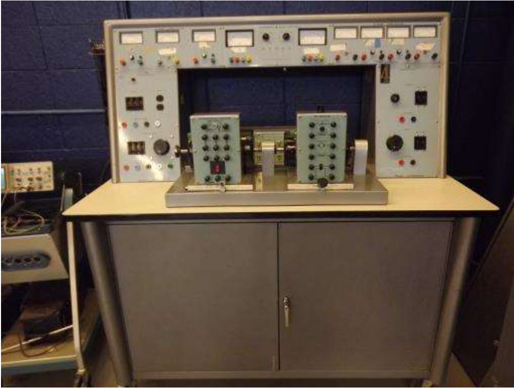
Figure 77: EPS / Motor Controls Training Bench
