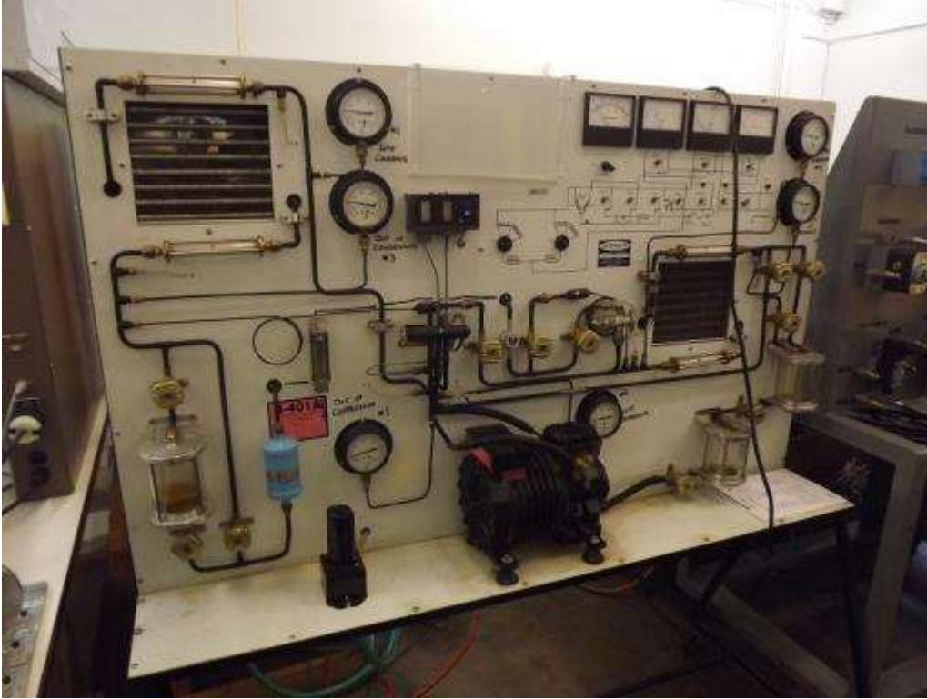
Figure 1: Refrigeration Cycle Test Bench
