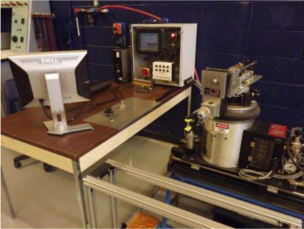
Figure 75: PLC controlled cylindrical robot
