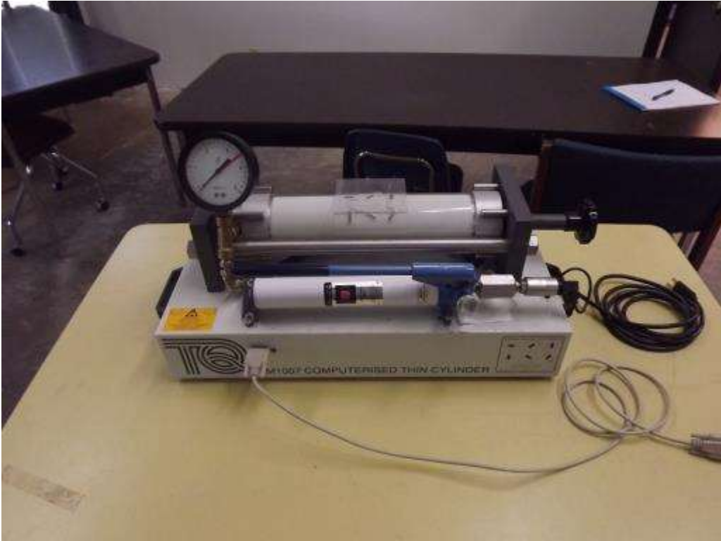
Figure 16: Computerized Pressure Vessel
