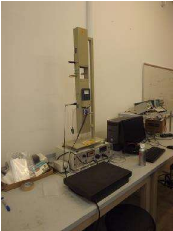
Figure 22: Convective Heat Transfer
