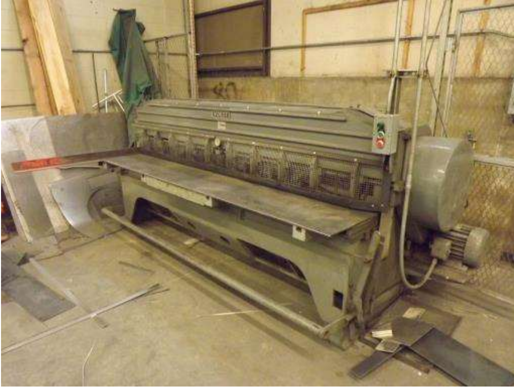
Figure 50: Voest Hi-Capacity Shear 1/8" Max
