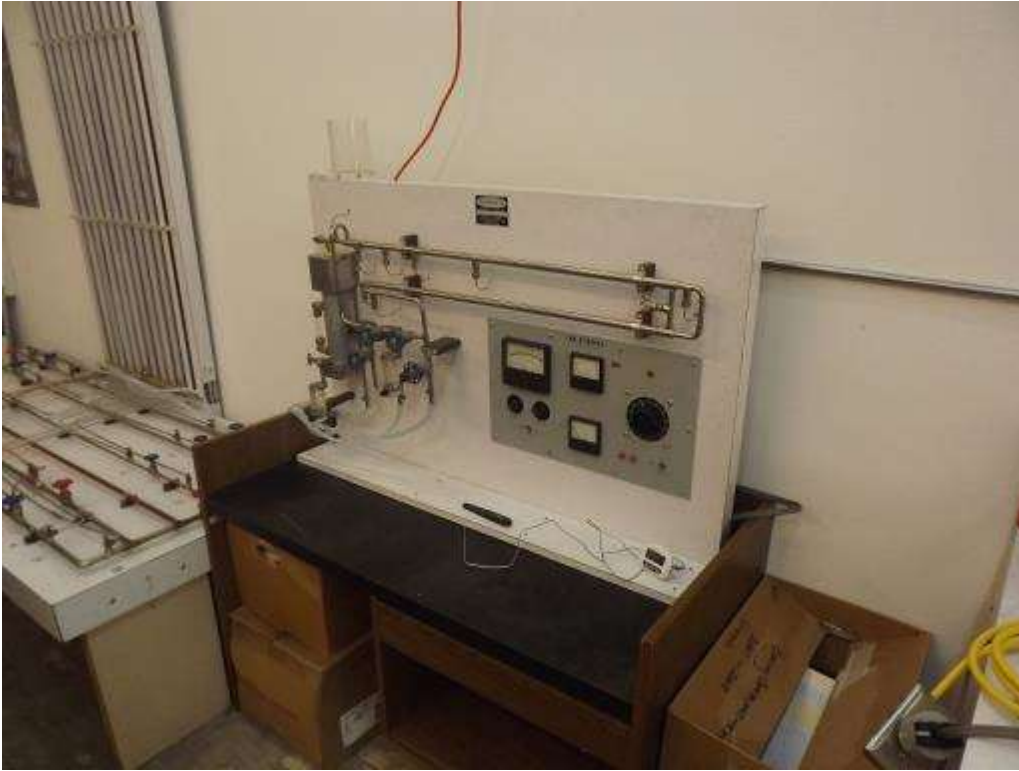
Figure 19: Tube in Tube Heat Exchanger
